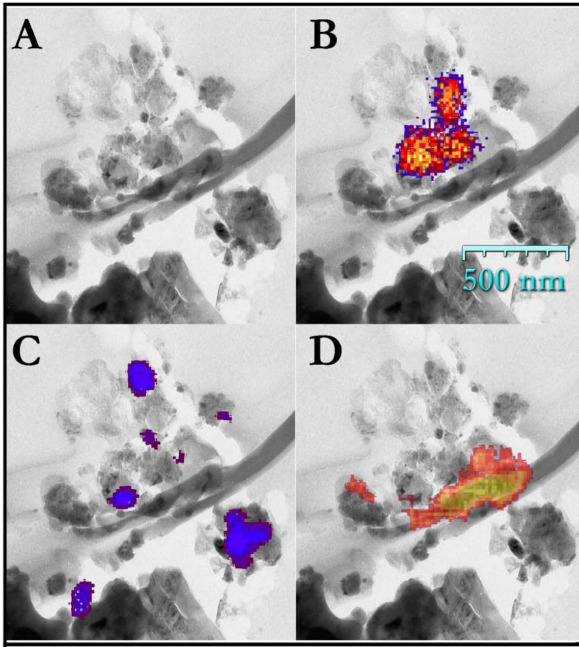
Figure 9: (A) TEM brightfield image of IDP L2011 B10A containing forsterite, enstatite, GEMS grains and carbonaceous matter. (B) Overlay of  $^{18}\text{O}$ -rich region identifying a supernova olivine grain. (C)  $^{32}\text{S}$  hotspots show the locations of FeS and GEMS grains (D)  $^{15}\text{N}$ -rich carbonaceous matter associated with presolar olivine grain. Messenger, Keller and Lauretta, 2005.
