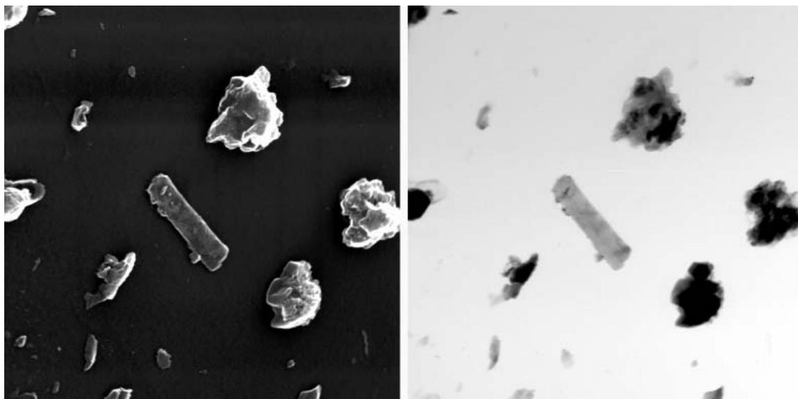
Figure 4: Individual submicron components mechanically separated from a CP interplanetary dust particle. On the left is a SEM image and a transmission image is on the right.
