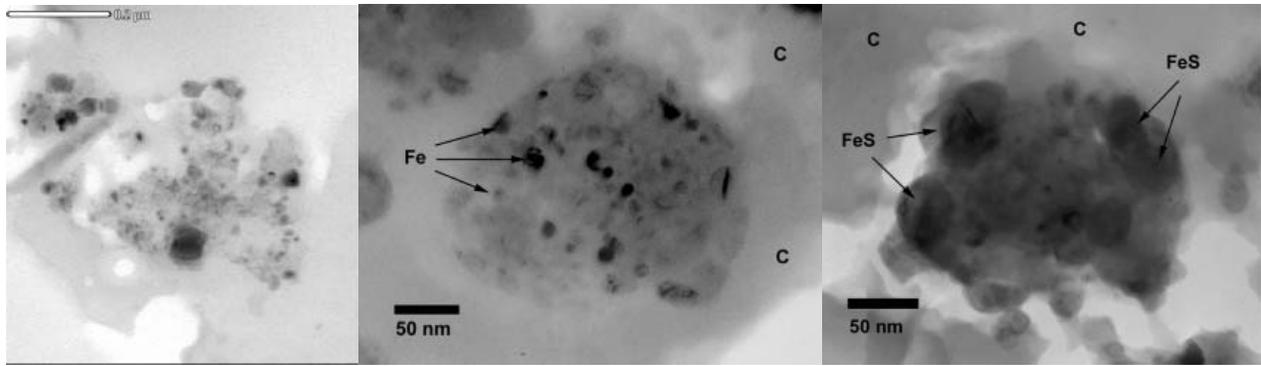
Figure 3: GEMS exhibit a diversity of compositions and morphologies, ranging from A: irregular grains, that may be a composite object (clump) (B): glass-rich GEMS grain (C): sulfide-rich GEMS grain.
