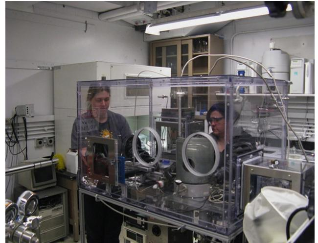
**Fig. 6.** The O/OREOS sample-fabrication-and-test facility for the flight sample cells at NASA Ames. Contained within a glove-box, this high-vacuum thin-film deposition system includes an Ocean Optics HR400CG-UV-vis spectrometer (200–1100 nm) for film characterization.
