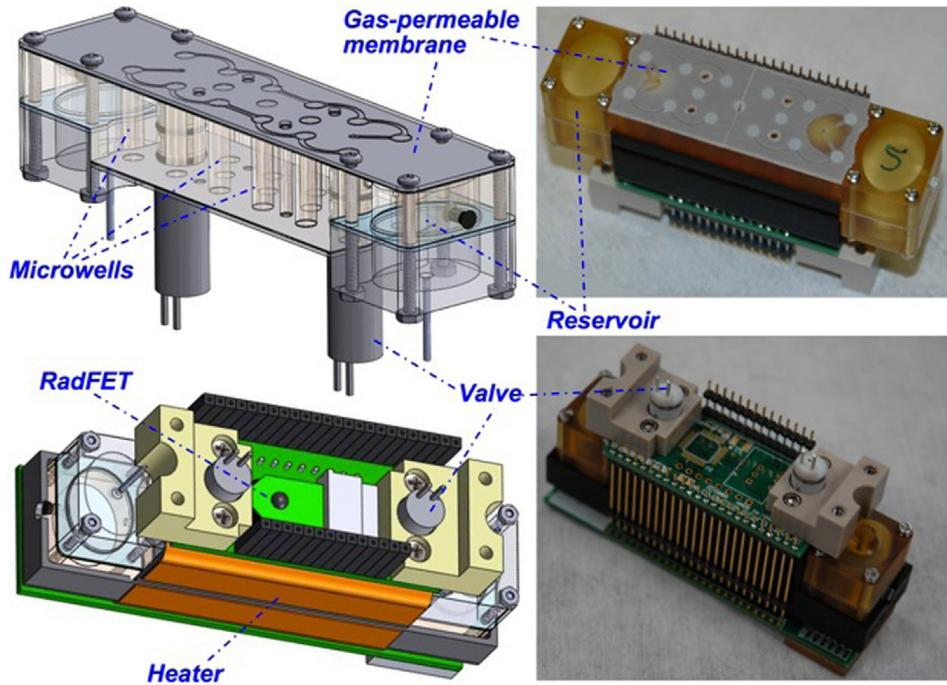
**Fig. 4.** Four different views (solid model at left, photographs at right) of one of three bioblocks included in the SESLO payload. The two valves protrude down from the block (upper left); reservoirs are the elliptical structures at both ends of the block; heater is orange and RadPET is a black dot near the center of the bottom left depiction. (For interpretation of the references to colour in this figure legend, the reader is referred to the web version of this article.)
