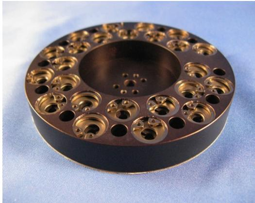
**Fig. 5.** The SEVO sample carousel holds 24 sample cells designed to expose organic thin films to both the full solar electromagnetic spectrum and the ionizing particle radiation of space. To measure the spectrum of a sample, the carousel, driven by a stepper motor, rotates the sample cell over an assembly of collection optics that focuses the transmitted light into an all-silica optical fiber which terminates into the compact UV-vis spectrometer.
