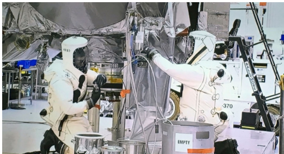
Fig. 17 Collection of flight hydrazine monopropellant for chemical and isotopic analysis
