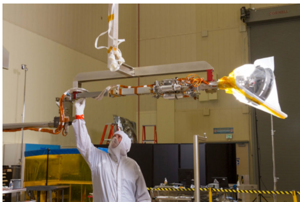
Fig. 4 Personnel properly gownned in the LM ISO 7 cleanroom and TAGSAM head protected by a PFTE bag
