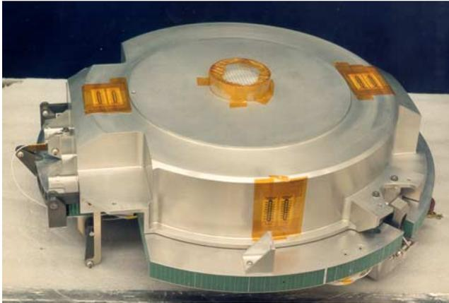
**Figure 9.** Photograph of the Sample Canister (SC), showing the base plate, the cover with center-mounted vent filter, and six of the eight temperature tapes.
