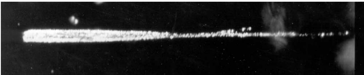
**Figure 4.** Intact capture in medium-density aerogel with the typical carrot track and with the particle lodged at the end of the track.
